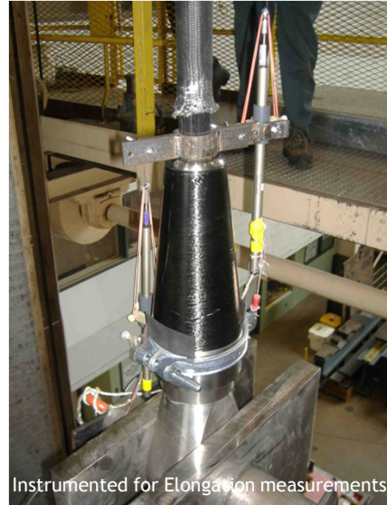
80tonne EC6 Cable in 5million pound test frame
