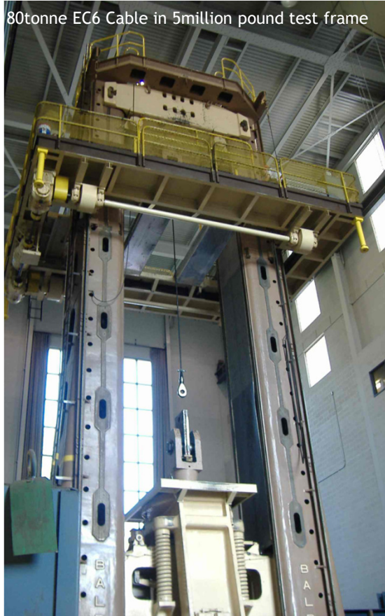
Instrumented for Elongation measurements
