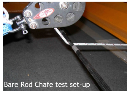
Instrumented for Elongation measurements
